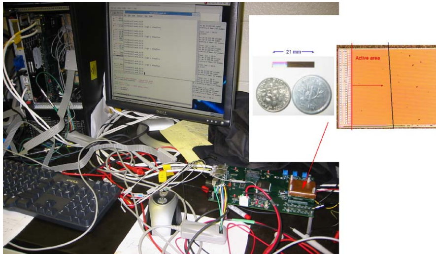
Fig. 3. Overview photo of a CAP3 test setup, with zoomed die views inset. The CAP3 die is reticle-size limited at about 21 mm in length and consists of 926 columns \times 128 rows of pixels, corresponding to just under 120 k pixels. Reading out at 10 kHz of triggered frame rates requires a throughput of over 1 Giga CDS pairs s^{-1} .
